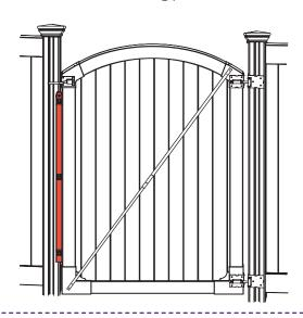
▶ The hinges can be adjusted moderately to bring the gate into level alignment with post.
